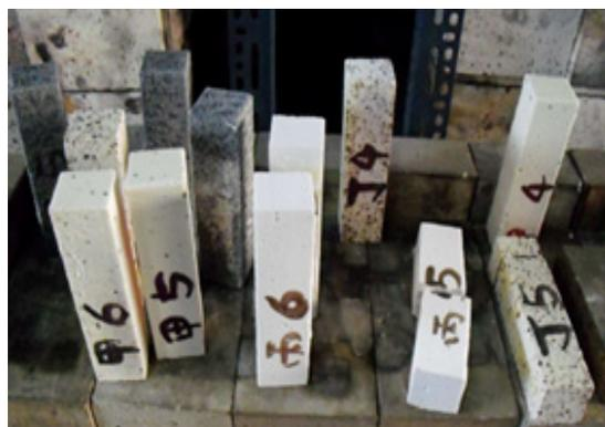
Fig.15. The thermal shock damage test for crucible refractories (left: heated, right: cold).
